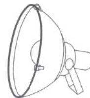
(a) Type A floodlight giving a symmetrical beam
