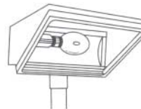
(c) Type C floodlight giving a fan-shaped beam with asymmetric distribution in the vertical plane
